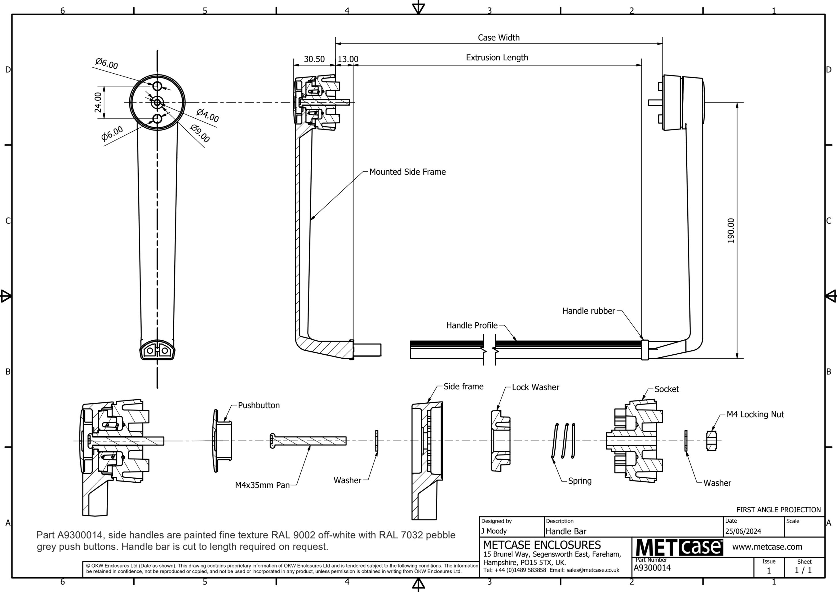
Part A9300014, side handles are painted fine texture RAL 9002 off-white with RAL 7032 pebble grey push buttons. Handle bar is cut to length required on request.
